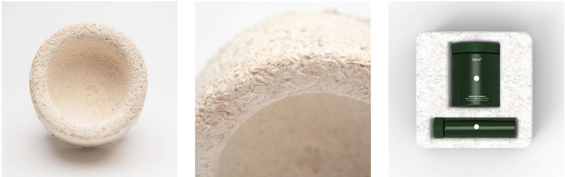
Fig 7. MycoComposit. A mycelium-based material used in packaging. (Credit: Paradise Packaging)
